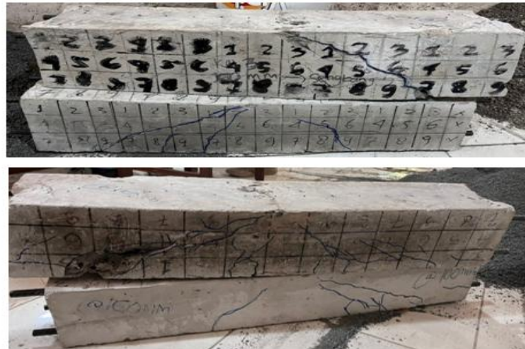
Figure 11. Front and Rear Views of Crack Patterns in Beams B1 and B2
