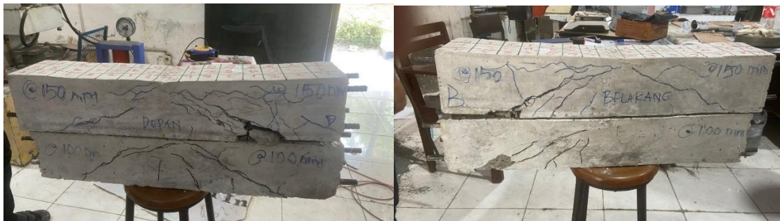
Figure 11. Front and Rear Views of Crack Patterns in Beams B3 and B4
