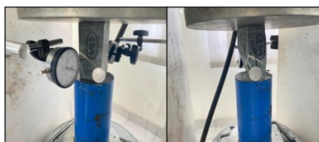
Figure 4 Testing of uniaxial compressive strength carried out on ST 09 samples of porphyry meta- andesite lithology
