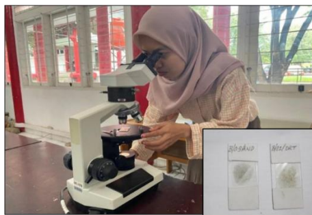
Figure 6 Petrographical investigation using a polarizing microscope
