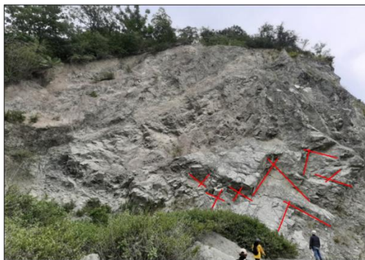
Figure 13. The appearance of a systematic joint structure found in the porphyritic andesite lithology at station 5 with a photo direction of N 23°E.
